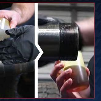
**Step 2** Apply a light coating of lubricant to the spindle surfaces.
